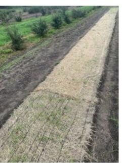
**Possible uses** The Paludi-mat consists of a Paludi fiber fleece, which is enclosed top and bottom in carrier nets made of jute. All components are sewn together with jute threads. Depending on the basis weight, the Paludi-mat serves as an erosion control mat (up to  $500 \text{ g/m}^2$ ) or as a fully organic mulch mat (from  $600 \text{ g/m}^2$ ) to suppress light-germinating grasses and plants.
