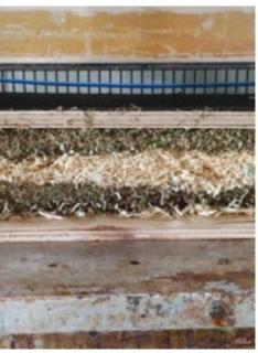
Possible uses This material can be used as plate material for indoor building. Research has shown that up to 75% of greater pond sedge (Carex riparia) can be incorporated without compromising the material's key properties. With a higher percentage of sedge edge, the mechanical properties decrease.
