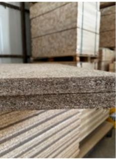
Possible uses Production of panels made from paludiculture sedge grass with a natural binder, suitable as infill material for interior doors.
