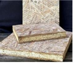
**Properties** Thermal conductivity value ( $\lambda$ ) of 0.083 W/mK at a density of 800 kg/m³ (measured by the University of Göttingen). Flammability test (small burner test, DIN 11925-2): after 15 seconds – 5 cm soot cone height; after 30 seconds – 6.5 cm (maximum allowable height: 15 cm). No afterglow. Provides a stiffening function comparable to typical OSB boards, but with improved fire protection and higher thermal insulation performance.
