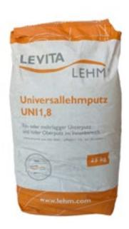
Possible uses "Lehmuniversalputz UNI 1.8" is a ready-to-use, dry clay plaster that can be applied both as a base coat and as a top coat. It consists of clay, loam, and washed mixed-grain sand (0-1.8 mm). It also contains almost invisible cattail fibers (Typha fibers), which provide excellent properties such as high strength, very low drying shrinkage (minimal cracking in thick layers), and very good moisture absorption and release.
